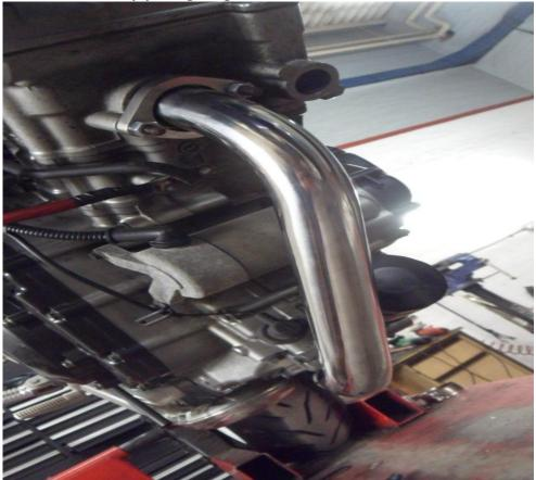
• Fit the L/H link pipe to the downpipe and mount to the frame.
