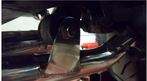
• Remove the pillion footrest brackets and re fit with the silencer mounts and spacers.
